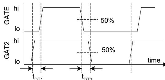
**Figure 2. GATE and GAT2 Timing and Phasing**
