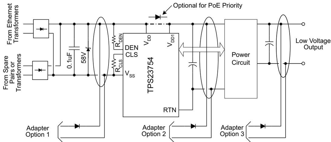
**Figure 23. ORing Configurations**
